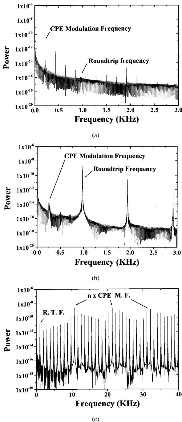
Fig. 4. Spectrum of lasing power. (a) Region I. (b) Region II. (c) Region III. Network span length 200 km. (CPE M. F.: Channel power equalizer modulation frequency. R. T. F.: round-trip frequency.)
