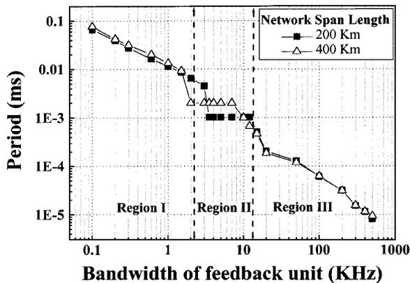
Fig. 2. Period of lasing power as a function of the bandwidth of the feedback circuit unit in a CPE (for single unit).
