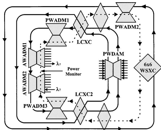
Fig. 1. Configuration of the MONET LEC-TB. The closed loop is marked with dashed lines (P-WADM: passive wavelength add/drop multiplexer; A-WADM: active wavelength add/drop multiplexer (the difference is whether or not it includes CPEs); LCXC: liquid crystal cross-connect; WSXC: wavelength selective cross-connect).
