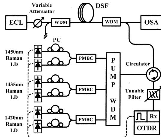
Fig. 1. Setup (ECL: tunable external cavity laser, PC: polarization controller, PMBC: polarization maintaining beam combiner).
