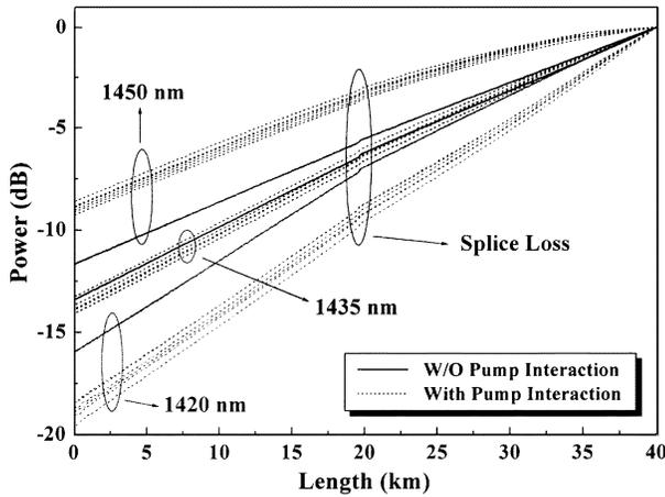
Fig. 2. Measured Raman pump evolution trace in the transmission fiber by p-OTDR (at different CW pump settings).
