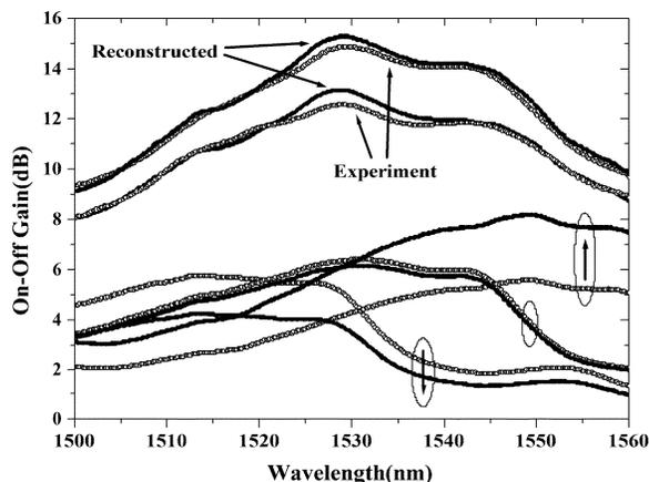
Fig. 3. Measured/reconstructed gain spectrum for single/multipump source (hollow: experiment, filled: reconstruction, pump power of 145/145/115 mW and 145/100/115 mW at 1420, 1435, 1450 nm, respectively).
