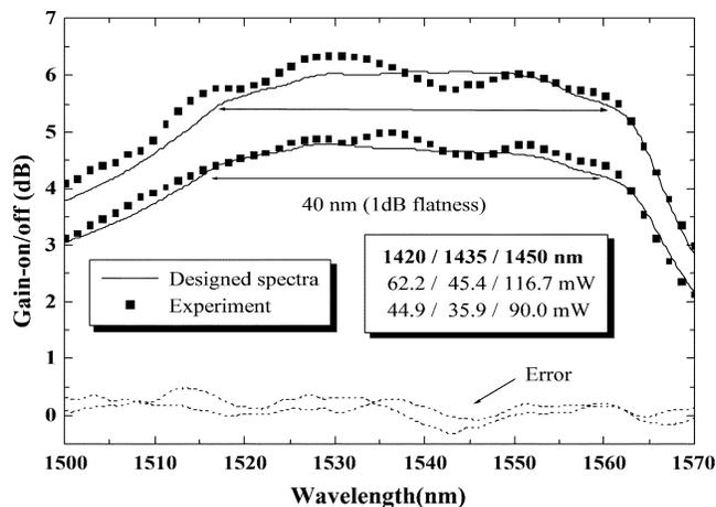
Fig. 4. Design constraints, designed target spectra, and experimentally measured Raman-gain spectrum.
