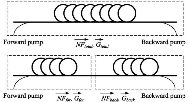
Fig. 1. Conceptual drawing for the construction of the design algorithm: distributed FRA and its equivalent, cascaded two-stage FRA.
