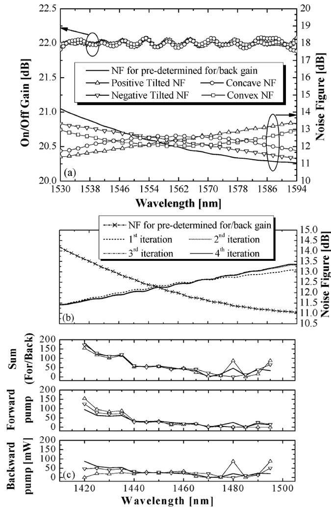
Fig. 3. FRA design (100-km DSF,  $P_S = -5$  dBm/ch, 22-dB ON-OFF gain,  $r = 0.6$ ). (a) NF achieved for different target spectra. (b) NF profiles at different stages of iteration. (c) Pump powers required for initial setting (solid line), and final stage of the NF design (+/- tilt:  $\Delta/\nabla$ ).
