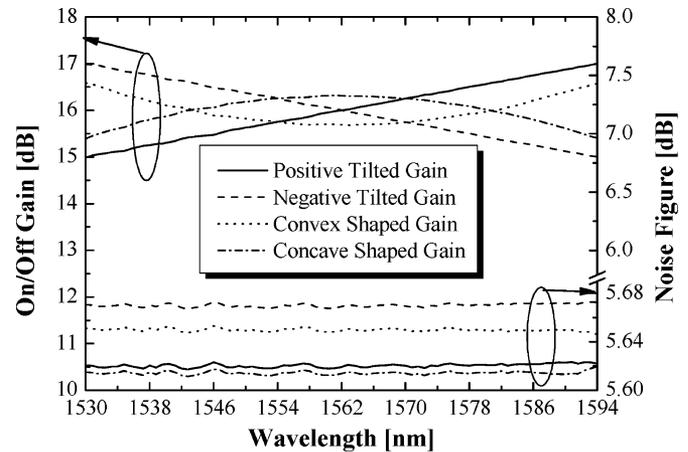
Fig. 4. Various gain shapes of a discrete FRA in the depletion regime (10-km DCF,  $P_S = -6$  dBm/ch,  $r = 0.7$ ), designed for flattened NF (pump wavelengths are identical to Fig. 3).
