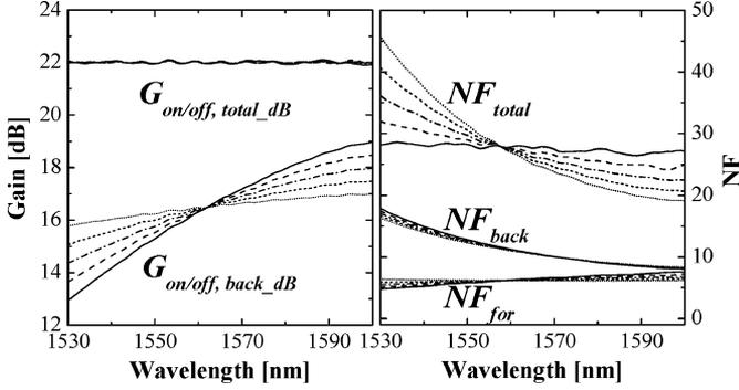
Fig. 2. Total, backward, and forward NF for various backward gain values (under the identical total gain of 22 dB).
